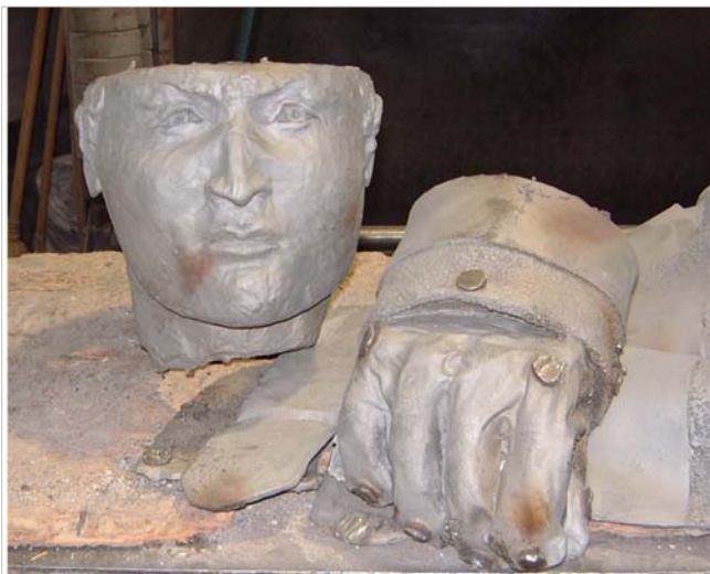
Cast Stainless Steel pieces of statues before assembly.
